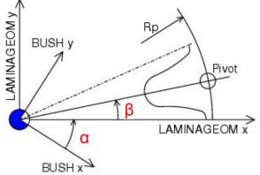
The pitch circle radius is used when wrapping the chain to define the radial position of the pivot point
