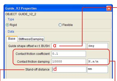
The stand-off distance is used only when wrapping the chain to define the distance between the face of the guide and the centre of the chain link
