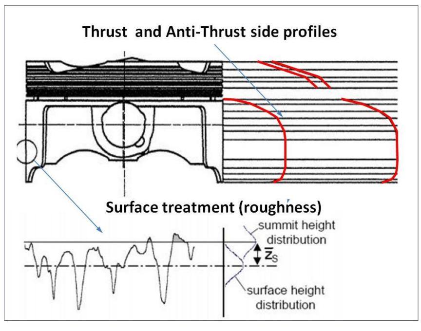
Pistons and cylinders are compliant and deformable due to thermal expansion as well as mutual interaction between the components. For this reasons, a thermal analysis using Finite Element (FE) methods often has to be performed. In this case, no CFD data for the thermal analysis was available, but Triumph kindly provided measured temperatures for the components instead.
