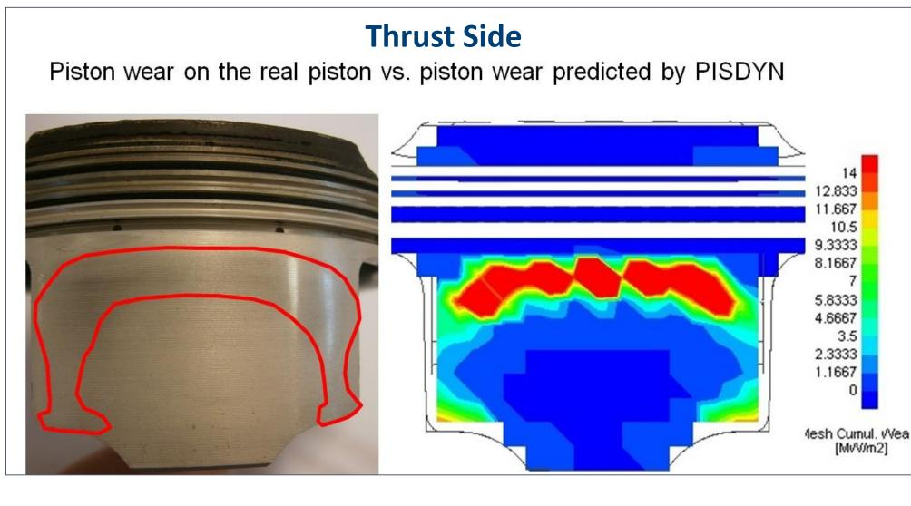
Engineering surfaces are not perfectly smooth. Often, pressure generated by hydrodynamic lubrication is not sufficient to prevent contact of asperities between the metallic surfaces. In this case, the asperity contact pressure is calculated using the Greenwood-Tripp model. This model considers cone shaped asperities with random heights.
